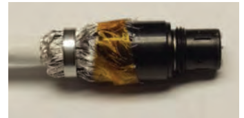
Figure 46: Attaching microband to socket
