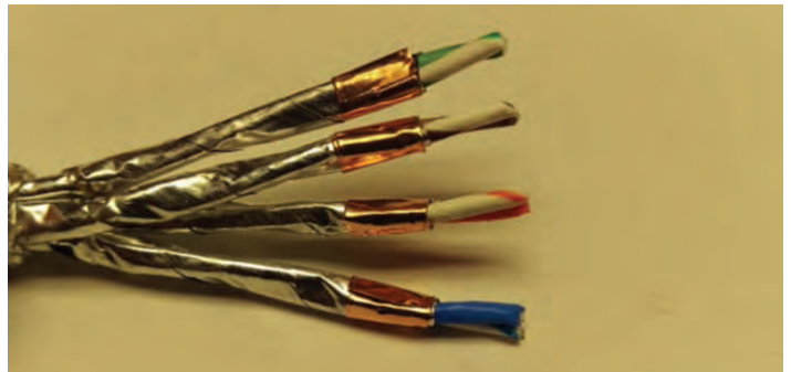
Figure 34: Removing the foil edge
