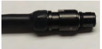
Figure 52: Shrinking tubing on socket backshell
