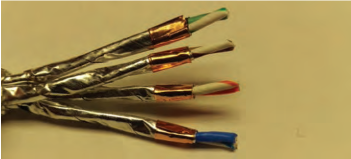
Figure 17: Removing the foil edge
