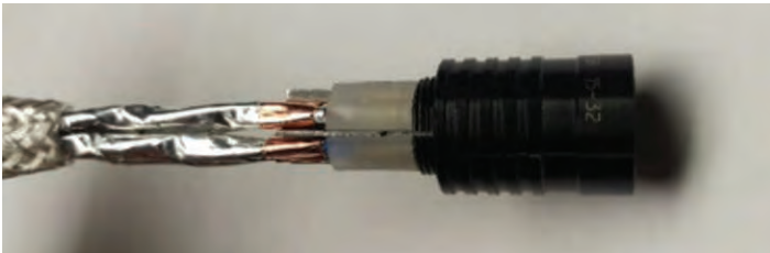
Figure 23: Inserting the back insulator
