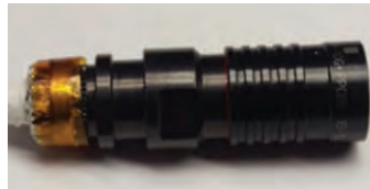
Figure 49: Taping microband on plug
