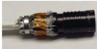
Figure 45: Attaching microband to plug
