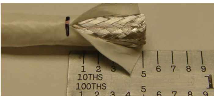
Figure 13: Slitting the cable jacket
