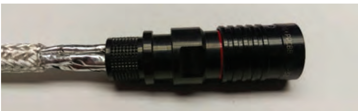
Figure 25: Seating the backshell
