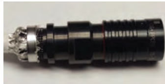
Figure 47: Trimming excess braid on plug
