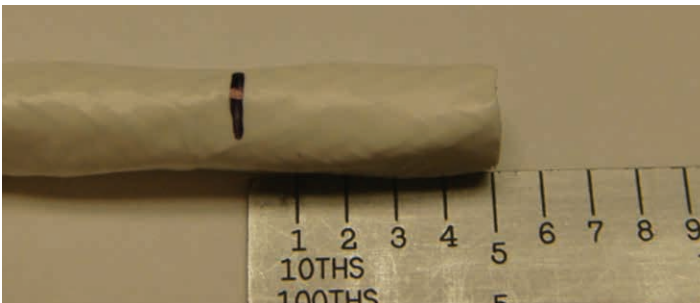
Figure 12: Marking the cable
