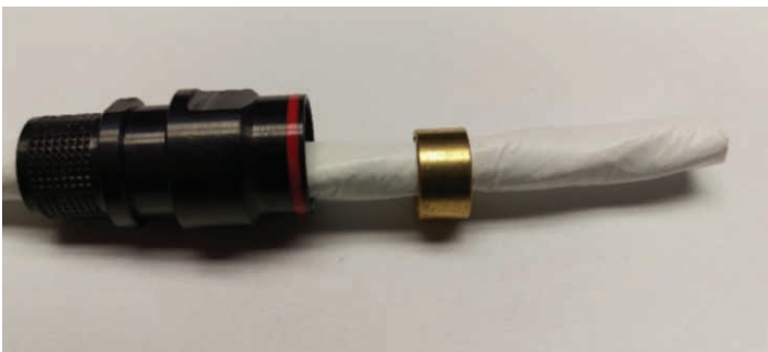
Figure 11: Sliding components onto the cable
