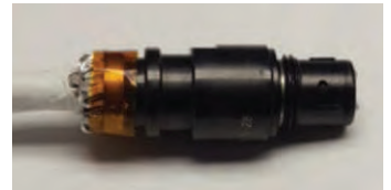
Figure 50: Taping microband on socket
